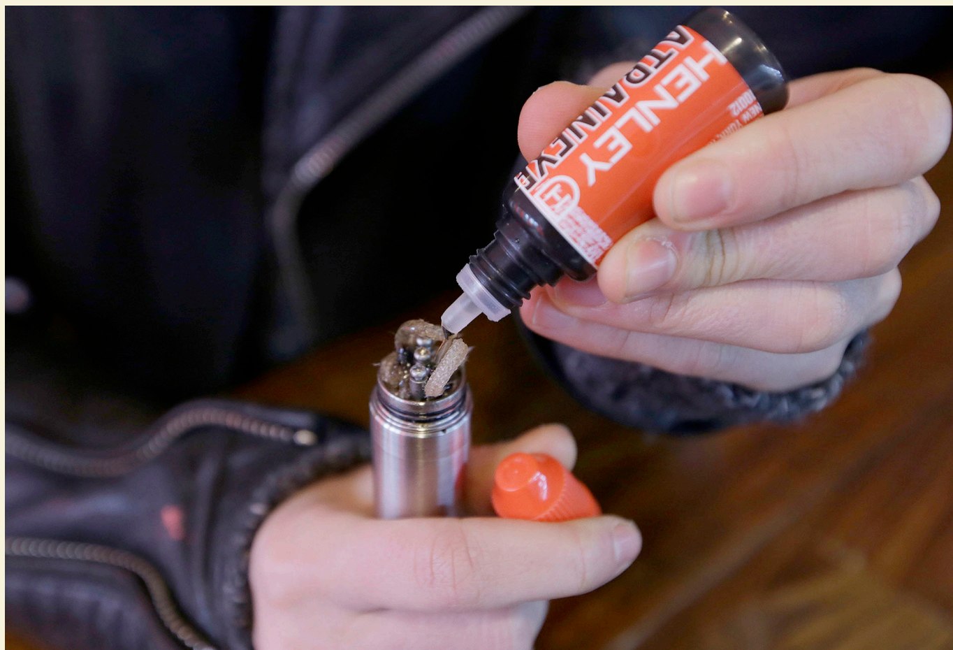
Although manufacturers offer many different designs of e-cigarettes, all involve the same basic concept: A heating element at one end aerosolizes a liquid nicotine solution, and the vapor is inhaled through a mouthpiece. © AP Photo/Frank Franklin II
